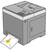
2 Remove the standard 250-sheet tray from the printer, and then pull out the jammed paper remaining inside the printer. If no jammed paper can be found or you are unable to remove the paper, go to the next step to remove the jammed paper from the inside of the printer.
